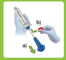
Retract the blue handle and remove the red plunger stop ring
